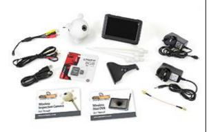
DVR main body User manual USB Cable AV-IN Cable AV-OUT Cable DVR Charger Back DVR holder FREE Mini SD card Antenna Switch Cable Instruction Manual
